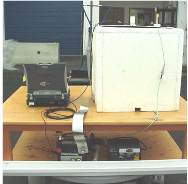
Photograph F.7-6 - Back of Radiated Emission Setup with vehicle-mount antenna and cradle
