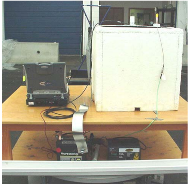
Photograph D.7-6 - Back of Radiated Emission Setup with vehicle-mount antenna and cradle
