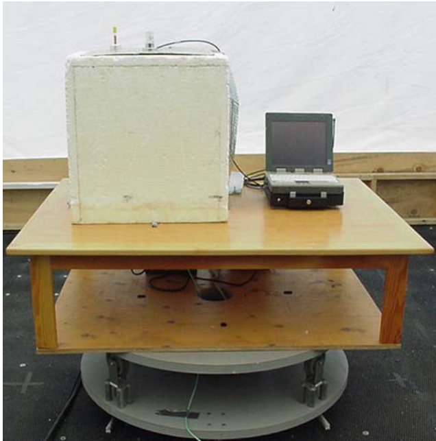
Photograph D.7-5 - Front of Radiated Emission Setup with vehicle-mount antenna and cradle
