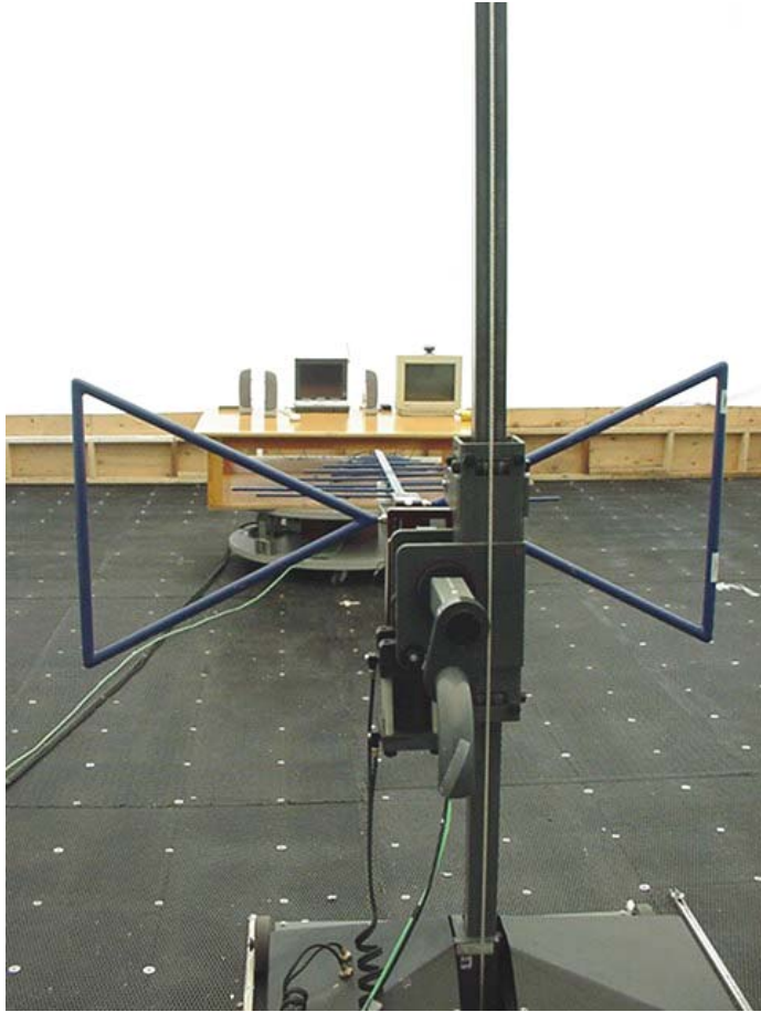
Photograph C.7-1 - DUT Swivel Dipole Antenna with Horizontal Bilog Receive Antenna Setup
