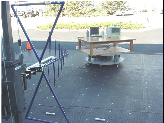
Photograph I-4 - Vertical Polarization (30MHz - 1 GHz)
