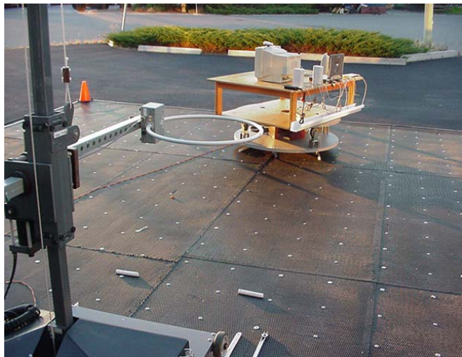
Photograph I-3 - Horizontal Polarization (30MHz - 1 GHz)
