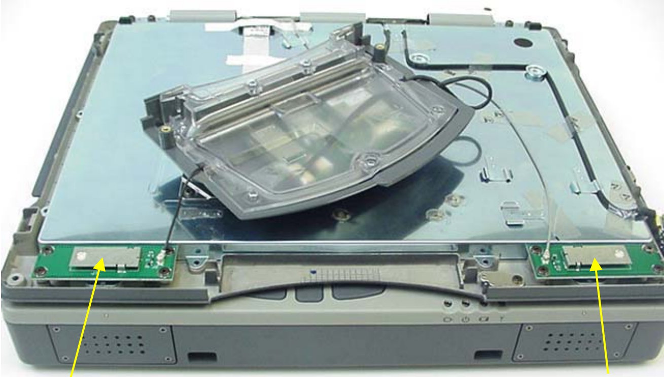
WLAN Surface-Mount Antenna (Upper Rear Right Side of LCD Display)
