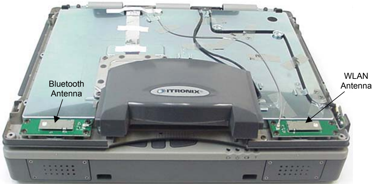
Photograph A-7 - Surface Mount Antenna Placement
