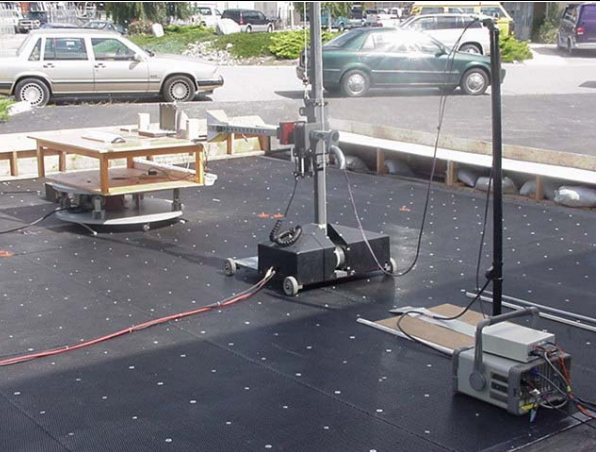
Photograph F-5 - 3115 Horn with LNA @ 1m
