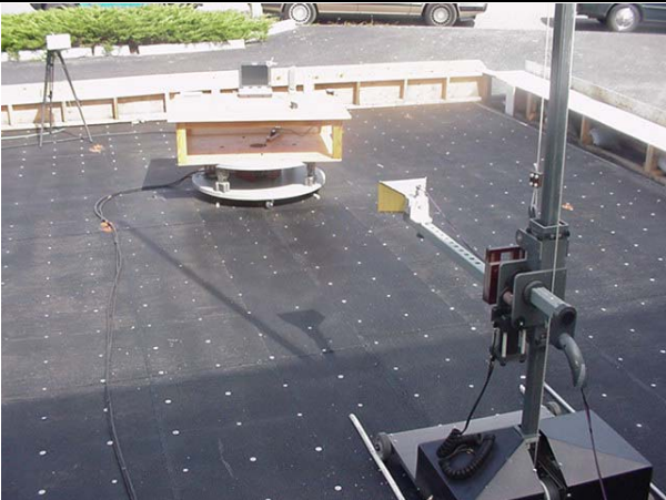
Photograph F-5 - 3115 Horn with LNA @ 1m
