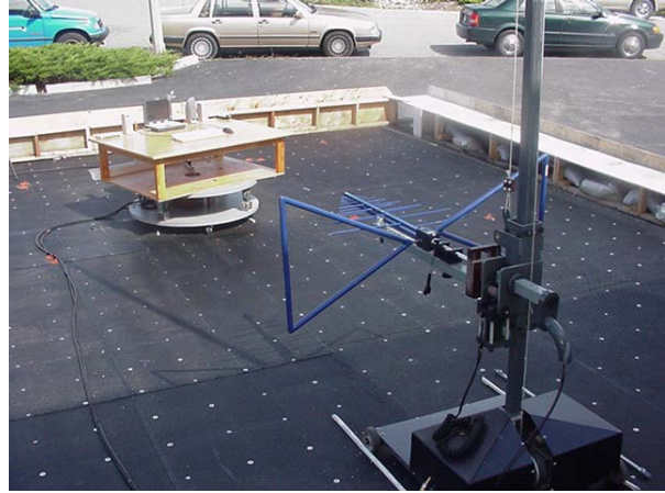
Photograph F-4 - 3115 Horn with LNA @ 3m
