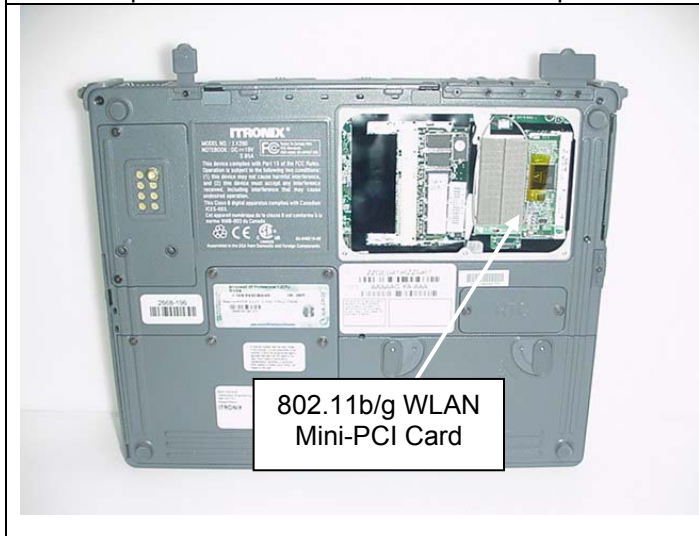
Photograph A-5 - Bottom of IX260+ Laptop PC with bottom panel removed to show WLAN card placement
