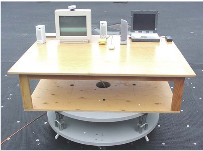
Photograph F-3 - Front of Radiated Emission Configuration
