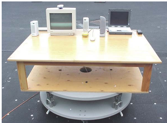
Photograph E-3 - Front of Radiated Emission Configuration
