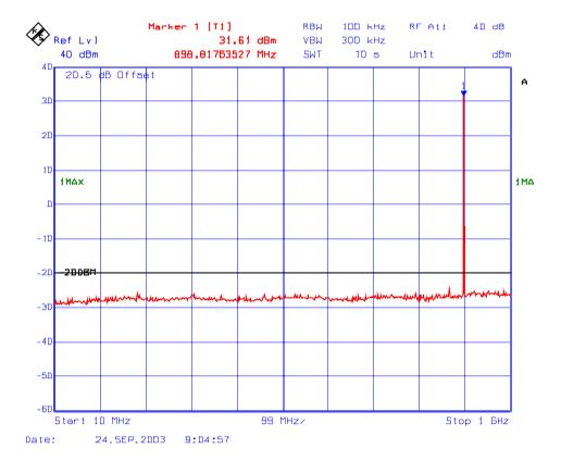
Plot # 14: Spurious Emission Conducted at Antenna terminal, High power setting Frequency: 898.5 MHz, Modulation: 2-Level 8kbps GMSK
