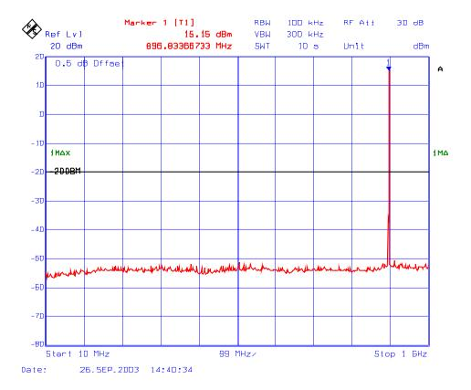
Plot # 18 : Spurious Emission Conducted at Antenna terminal, Low power setting Frequency: 896 MHz, Modulation: 2-Level 8kbps GMSK
