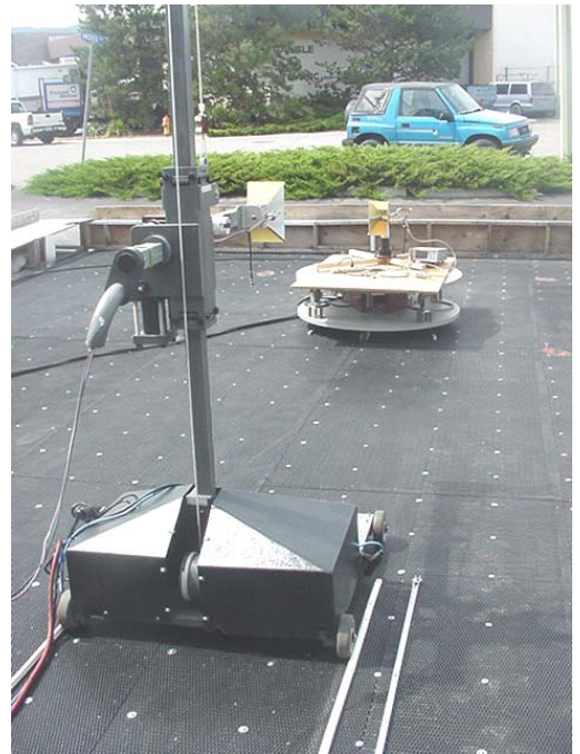
Photograph B.7-4 - Horn Substitution Setup
