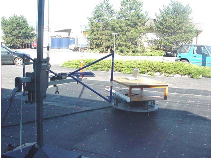
Photograph B.7-3 - Dipole Substitution Setup
