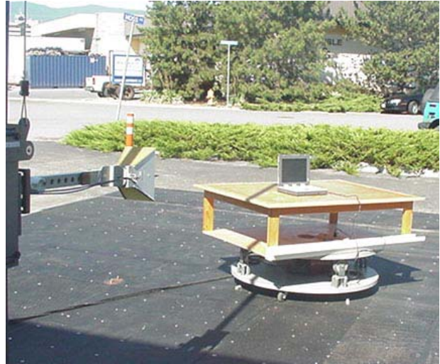
Photograph B.7-4 - Horn Substitution Setup
