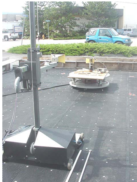
Photograph B.7-8 - Horn Substitution Setup
