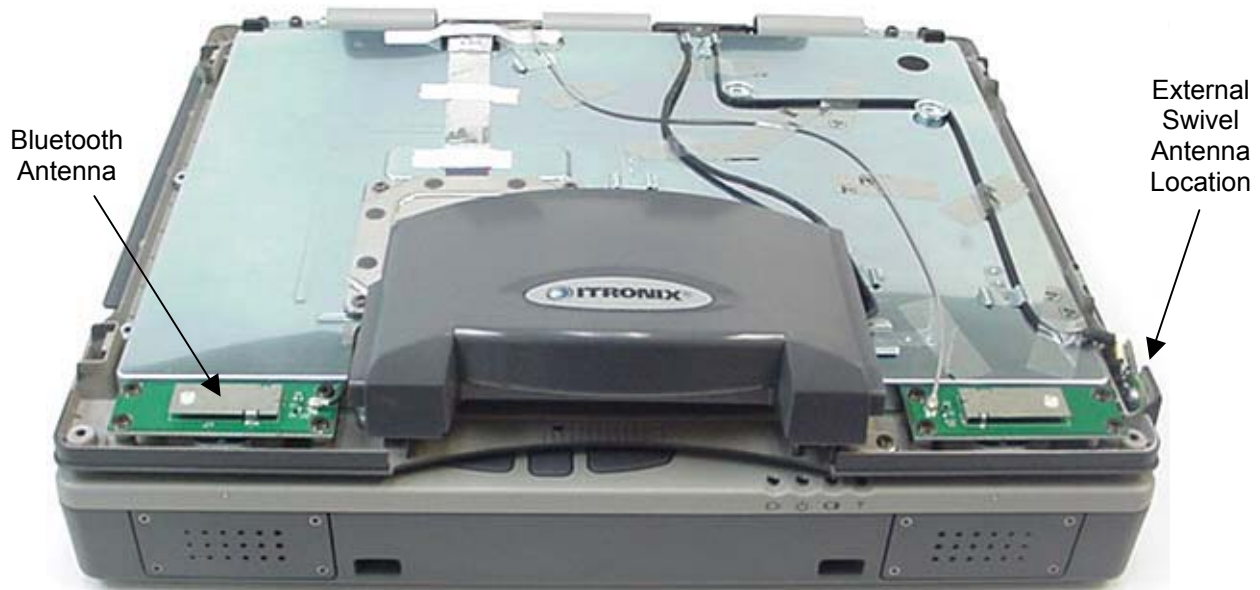
Photograph A-7 –Surface-Mount Antenna Placement
