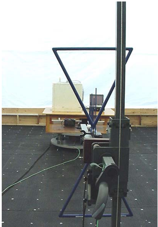
Photograph C.7-2 - DUT Vehicle Antenna & Cradle with Vertical Bilog Receive Antenna Setup
