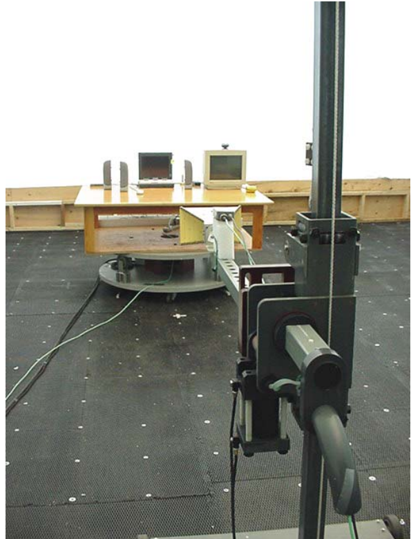
Photograph F.7-4 - Front of Radiated Emission Setup with vehicle-mount antenna and cradle
