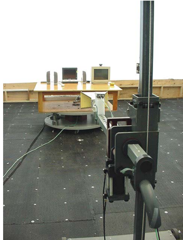
Photograph D.7-4 - Back of Radiated Emission Setup
