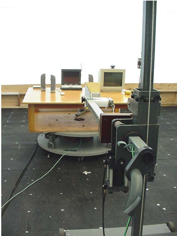
Photograph D.7-3 - Front of Radiated Emission Setup
