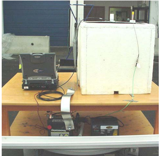
Photograph D.7-6 - Back of Radiated Emission Setup with vehicle-mount antenna and cradle
