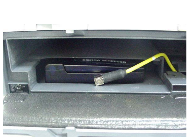
Photograph A.1-6 - CDMA Modem installed in DUT
