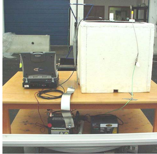
Photograph E.7-6 - Back of Radiated Emission Setup with vehicle-mount antenna and cradle
