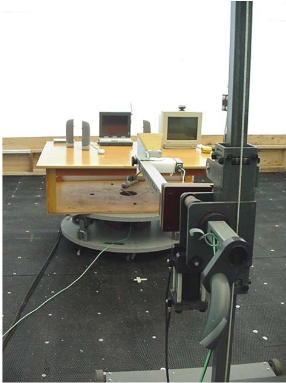
Photograph F.7-3 - Back of Radiated Emission Setup with attached swivel dipole antenna
