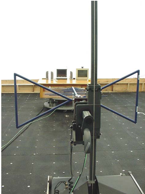
Photograph C.7-2 - Front of Radiated Emission Setup
