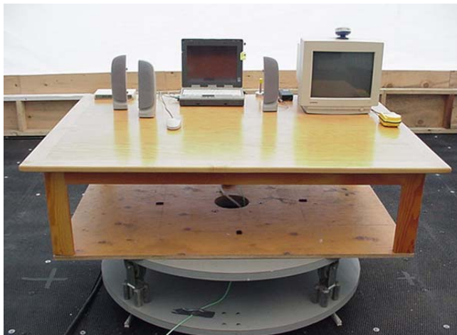
Photograph F.7-3 - Front of Radiated Emission Setup
