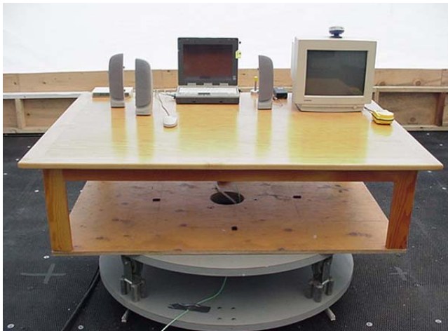
Photograph E.7-3 - Front of Radiated Emission Setup
