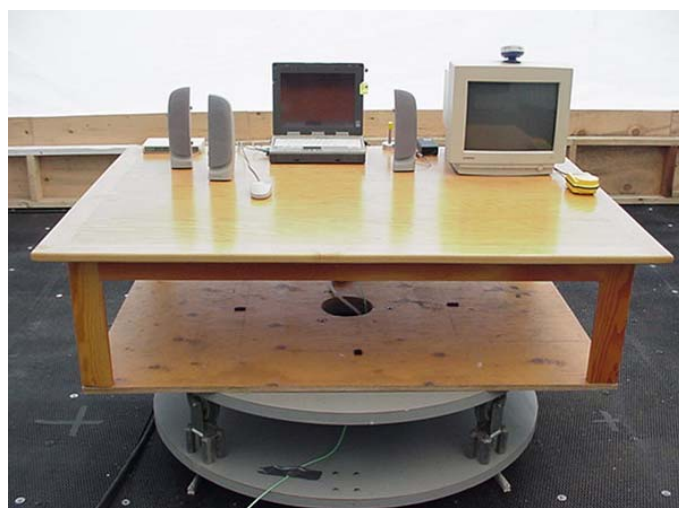
Photograph C.7-2 - Front of Radiated Emission Setup
