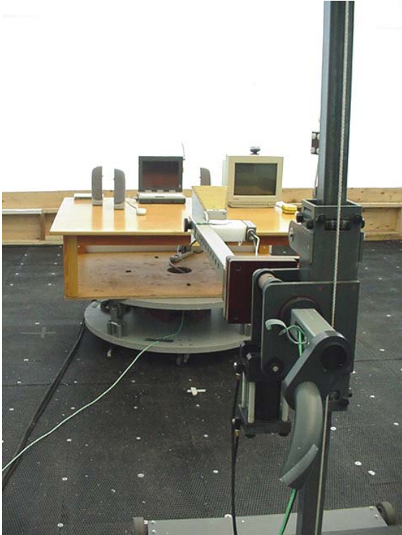
Photograph D.7-3 - Front of Radiated Emission Setup
