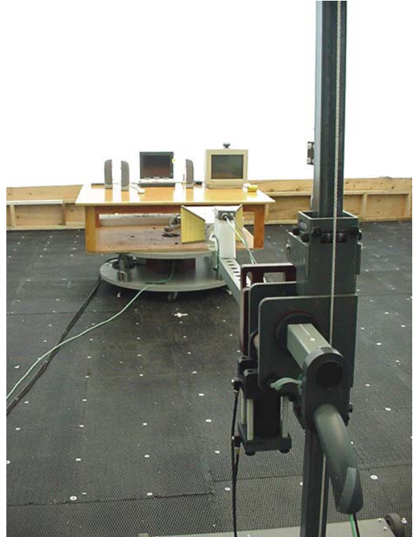
Photograph D.7-4 - Back of Radiated Emission Setup
