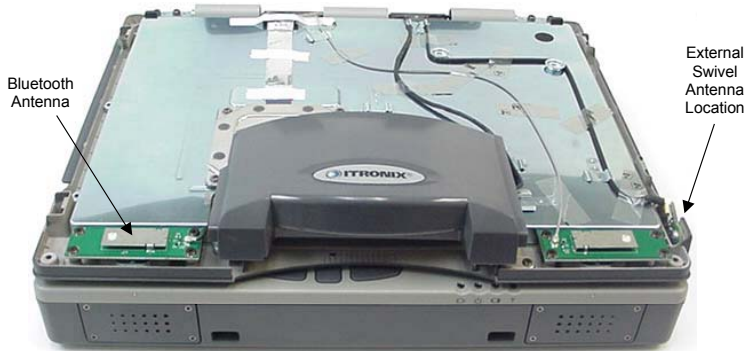
Photograph A.1-5 - CDMA and Bluetooth Antenna Locations
