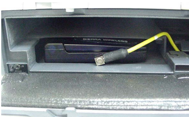
Photograph A.1-7 - CDMA Modem installed in PC
