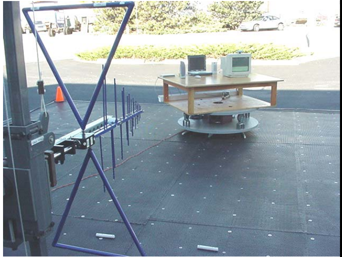
Photograph I-4 - Vertical Polarization (30MHz - 1 GHz)
