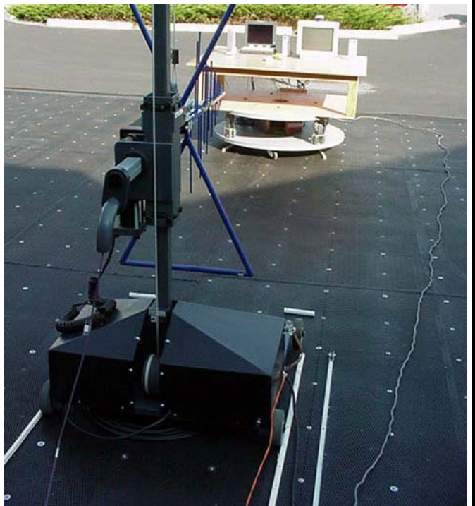
Photograph I-4 - Vertical Polarization (30MHz - 1 GHz)
