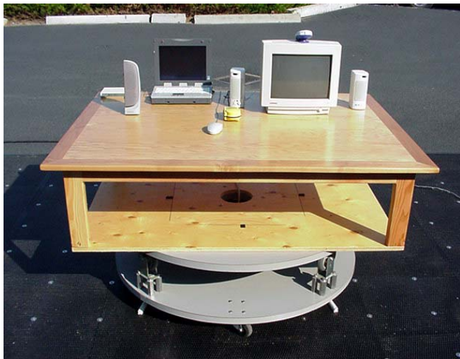
Photograph I-5 - Front of Radiated Emission Configuration
