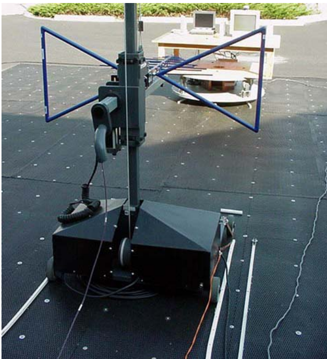
Photograph I-3 - Horizontal Polarization (30MHz - 1 GHz)
