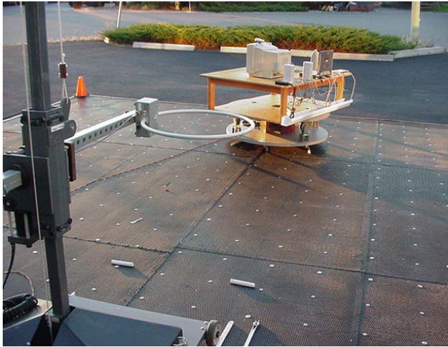
Photograph I-3 - Horizontal Polarization (30MHz - 1 GHz)
