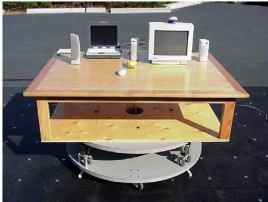
Photograph H-2 - Front of Radiated Emission Configuration
