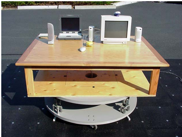
Photograph E-2 - Front of Radiated Emission Configuration
