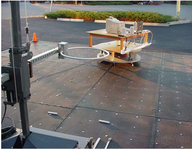
Photograph I-3 – Horizontal Polarization (30MHz – 1 GHz)
