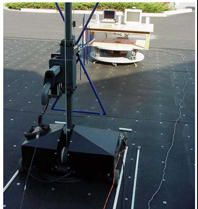
Photograph I-4 - Vertical Polarization (30MHz – 1 GHz)
