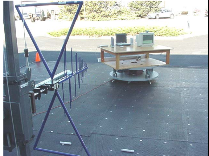
Photograph I-4 - Vertical Polarization (30MHz – 1 GHz)
