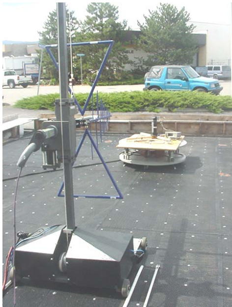
Photograph B.7-7 - Dipole Substitution Setup
