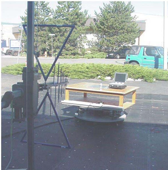
Photograph B.7-7 - Dipole Substitution Setup
