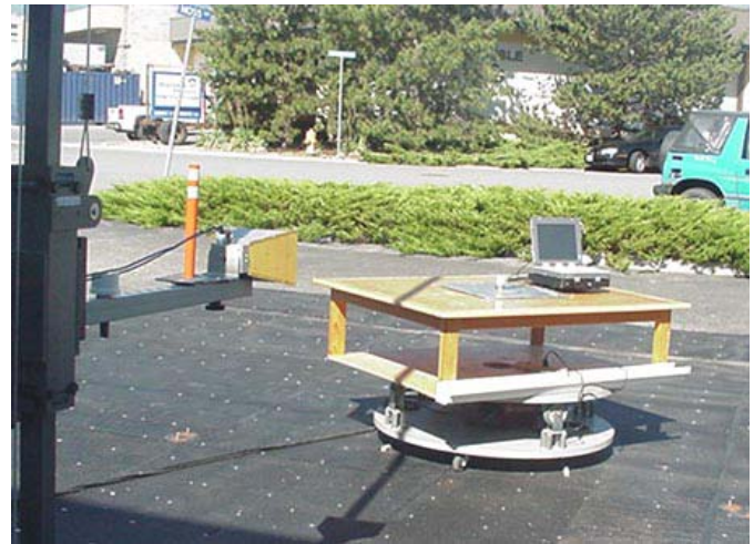
Photograph B.7-6 - Horn Receive Antenna with DUT Vehicle-Mount Antenna Configuration
