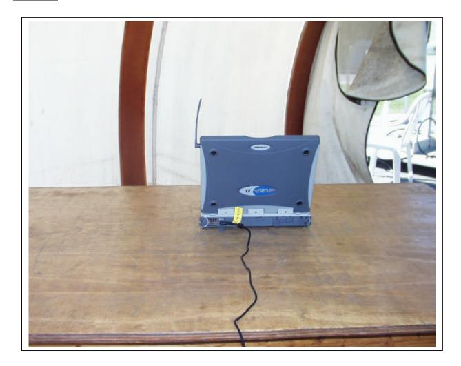
EUT: LAPTOP SYSTEM W/ BUILT-IN 850/1900MHz DUAL BAND GSM CARD
