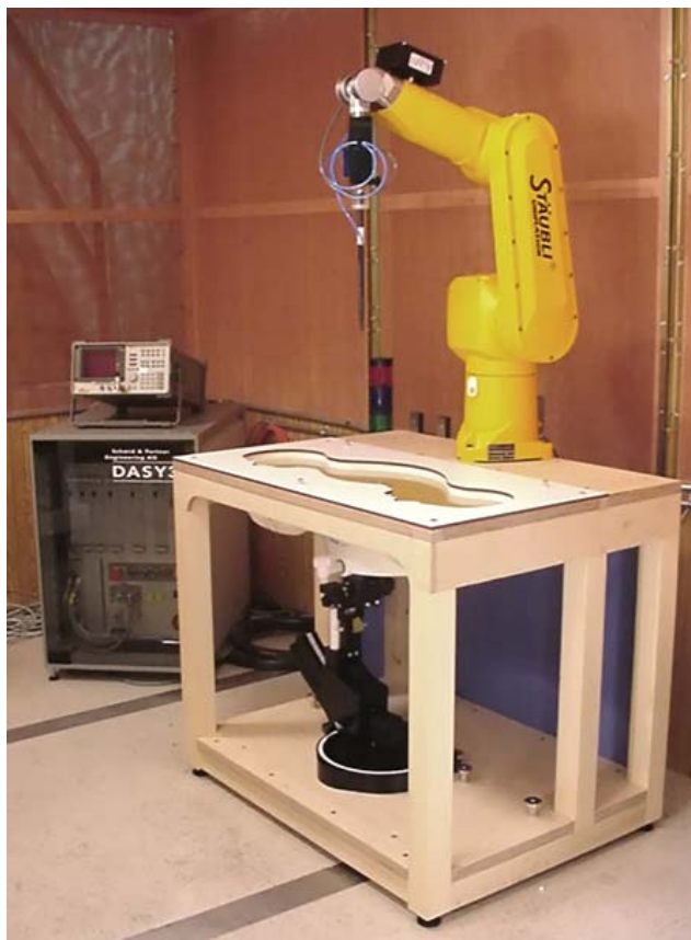
DASY3 SAR Measurement System with SAM phantom
