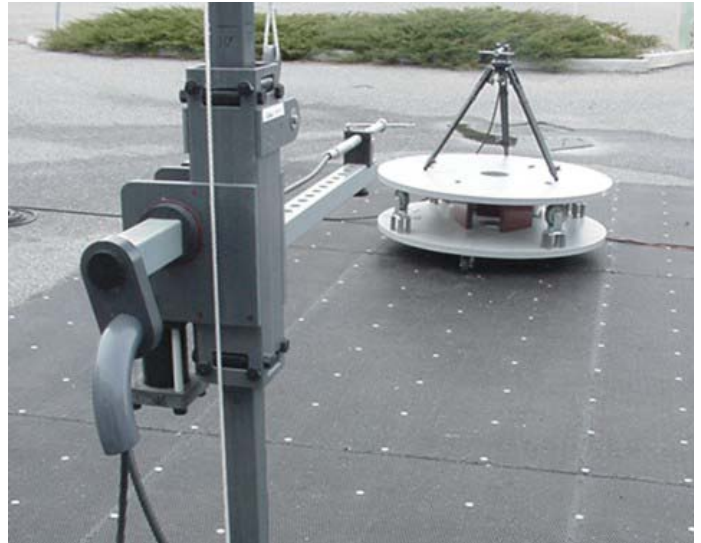
Signal Substitution Test Setup Photograph - Dipole Antenna
