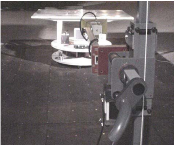
Radiated Measurement Test Setup Photograph - Horn Antenna
