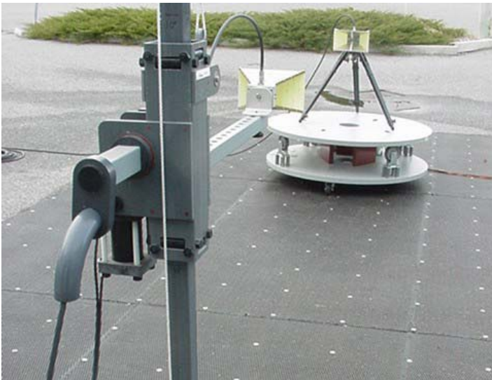
Signal Substitution Test Setup Photograph - Horn Antenna
