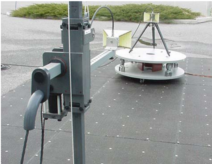
Signal Substitution Test Setup Photograph - Horn Antenna
