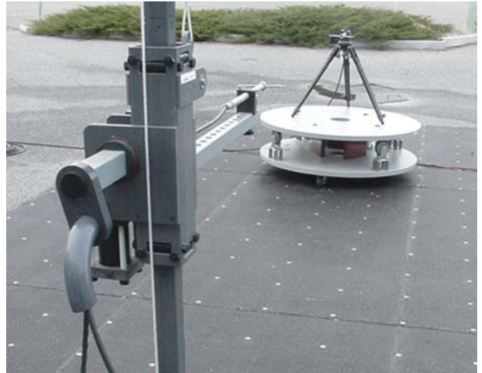
Signal Substitution Test Setup Photograph - Dipole Antenna
