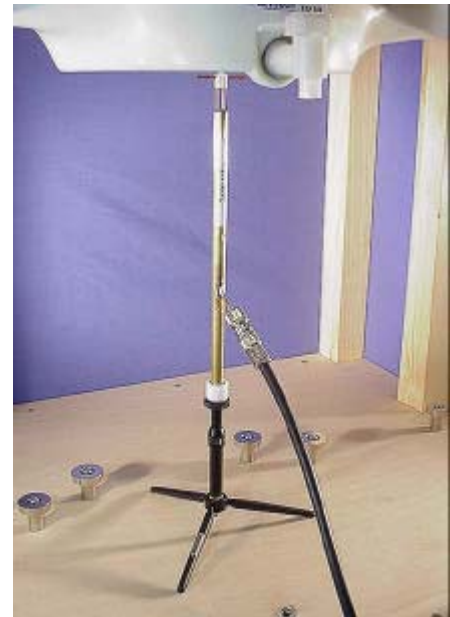
2450MHz System Check Setup Photograph
