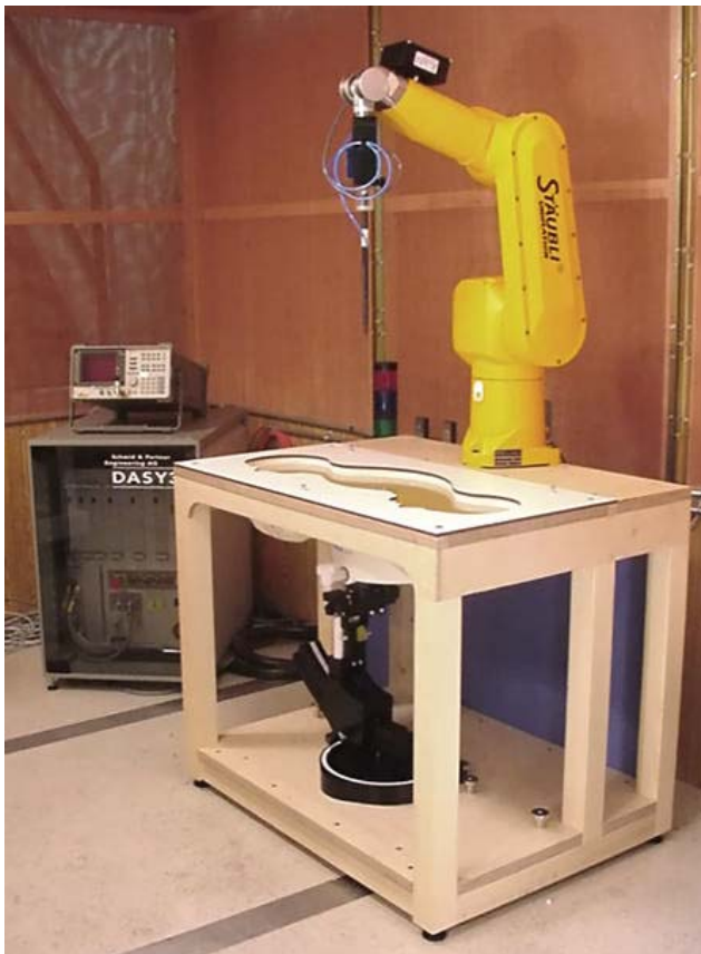
DASY3 SAR Measurement System with SAM phantom
