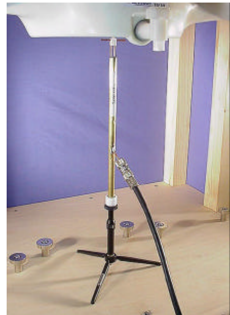
2450MHz System Check Setup Photograph
