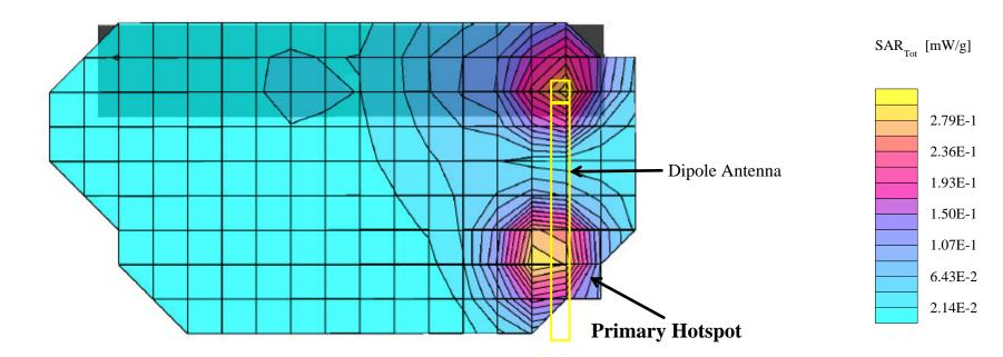
$\begin{array}{l} \mbox{Itronix Corporation FCC ID: KBCIX260AC750-MPI} \\ & SAM \mbox{Phantom; Flat Section; Position: (90°,0°)} \\ \mbox{Probe: ET3DV6 - SN1387; ConvF(4.90,4.90,4.90); Crest factor: 2.0} \\ & 1900 \mbox{ MHz Muscle: } \sigma = 1.55 \mbox{ mho/m } \epsilon_r = 51.1 \mbox{ } \rho = 1.00 \mbox{ g/cm}^3 \\ & Coarse: \mbox{ Dx = 15.0, Dy = 15.0, Dz = 10.0} \\ & Cube \mbox{ } 5x5x7 \\ & SAR \mbox{ } (1g): \mbox{ } 0.221 \mbox{ mW/g, SAR (10g): 0.129 \mbox{ mW/g}} \end{array}$
