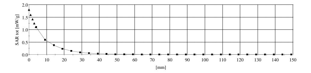
$\begin{array}{l} \mbox{Itronix Corporation FCC ID: KBCIX260AC750-MPI} \\ \mbox{SAM Phantom; Flat Section; Position: (90°,0°)} \\ \mbox{Probe: ET3DV6 - SN1387; ConvF(4.90,4.90,4.90); Crest factor: 2.0} \\ \mbox{1900 MHz Muscle: } \sigma = 1.55 \mbox{ mho/m } \epsilon_r = 51.1 \ \rho = 1.00 \ g/cm^3 \\ \mbox{Coarse: } Dx = 15.0, Dy = 15.0, Dz = 10.0 \\ \mbox{Cube } 5x5x7 \\ \mbox{SAR (1g): 0.408 mW/g, SAR (10g): 0.215 mW/g} \end{array}$
