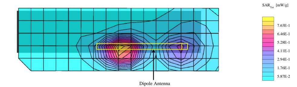
$\begin{array}{c} \mbox{Itronix Corporation FCC ID: KBCIX260AC750-MPI} \\ & SAM \mbox{Phantom; Flat Section; Position: (90°,0°)} \\ \mbox{Probe: ET3DV6 - SN1387; ConvF(4.90,4.90,4.90); Crest factor: 2.0} \\ & 1900 \mbox{ MHz Muscle: } \sigma = 1.55 \mbox{ mho}/m \ \epsilon_r = 51.1 \ \rho = 1.00 \ g/cm^3 \\ & Coarse: \mbox{Dx} = 15.0, \ \mbox{Dy} = 15.0, \ \mbox{Dz} = 10.0 \\ & Cube \ 5x5x7 \\ & SAR \ (1g): \ 0.886 \ \ mW/g, \ SAR \ (10g): \ 0.470 \ \ mW/g \end{array}$
