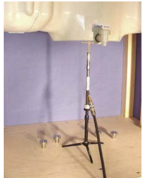
1800MHz System Check Setup Photograph
