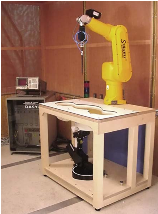
DASY3 SAR Measurement System with SAM phantom
