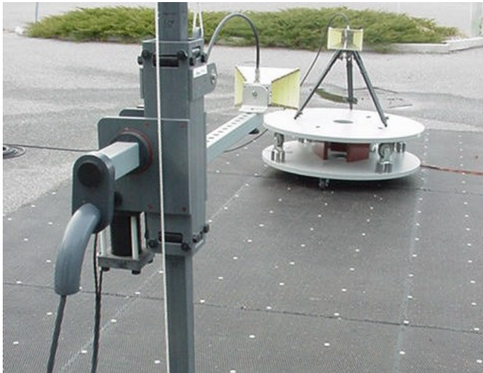
Signal Substitution Test Setup Photograph - Horn Antenna
