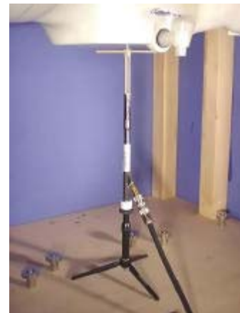
900MHz System Check Setup
