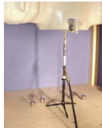
1800MHz System Check Setup
