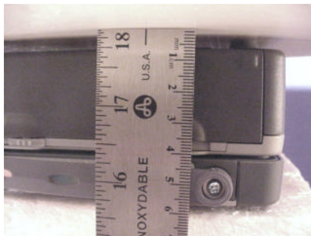
Distance from closest point of whip antenna feed/swivel to flat phantom - Bottom of PC
