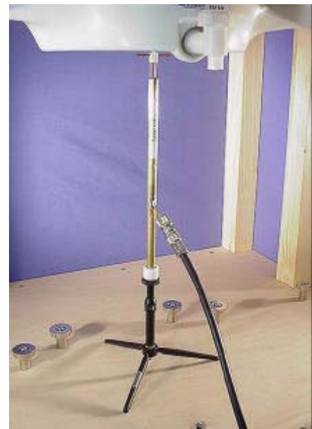
2450MHz System Check Setup Photograph
