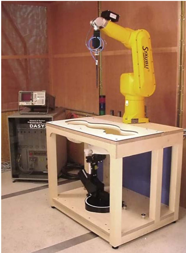
DASY3 SAR Measurement System with SAM phantom
