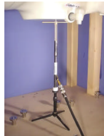
900MHz System Check Setup
