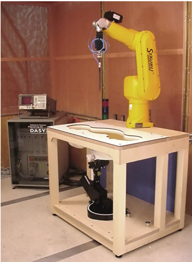
DASY3 SAR Measurement System with SAM phantom
