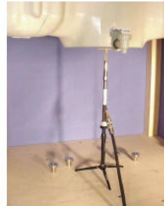
1800MHz System Check Setup
