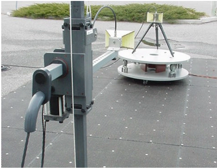
Signal Substitution Test Setup Photograph - Horn Antenna
