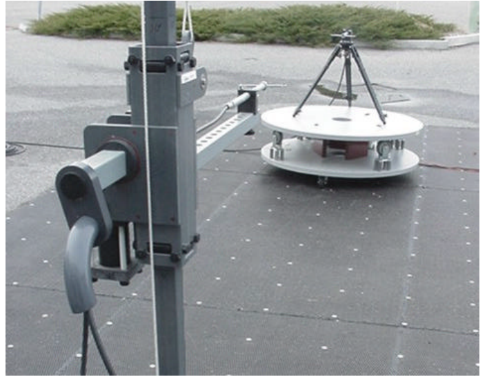
Signal Substitution Test Setup Photograph - Dipole Antenna
