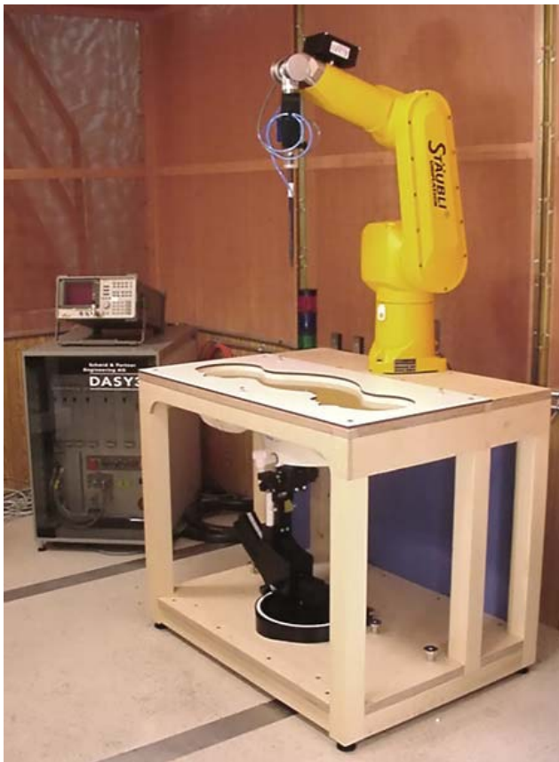
DASY3 SAR Measurement System with SAM phantom
