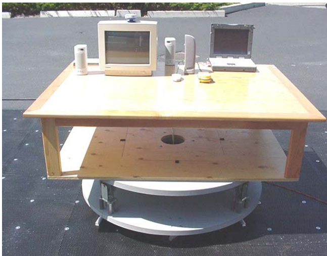
Photograph E-3 - Front of Radiated Emission Configuration
