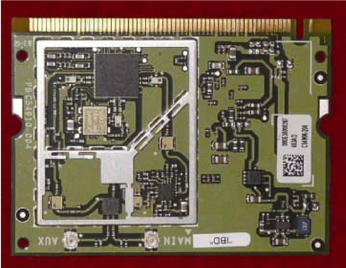
Front with Shielding Removed
