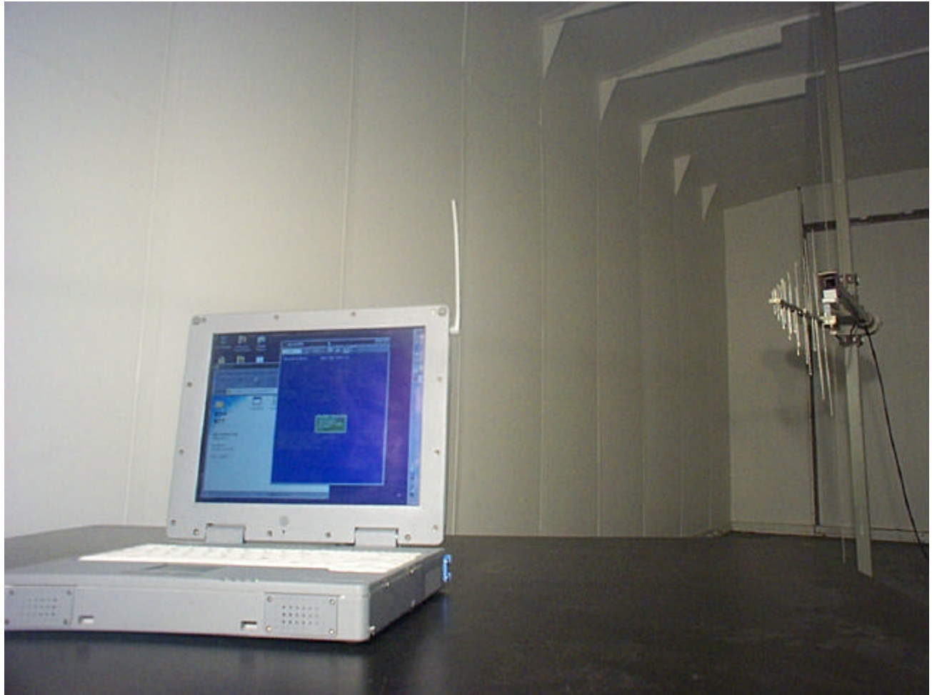
Spurious Emissions set up in OATS
