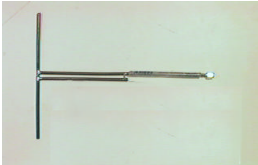
Reference Dipole Antenna Used for ERP Measurement
