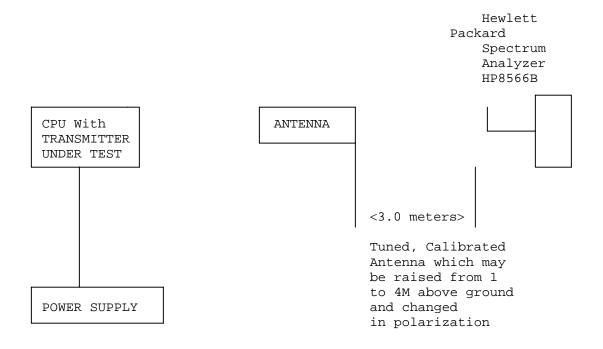
Equipment placed 80cm above ground on a rotatable platform.
