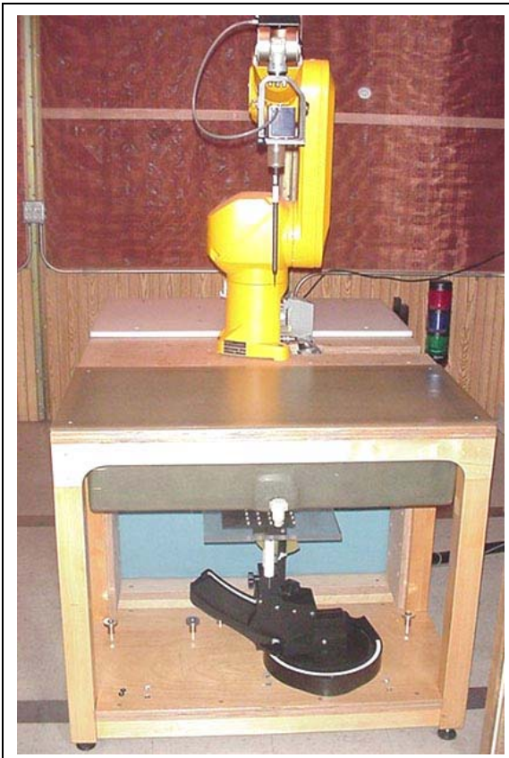
DASY4 SAR Measurement System with planar phantom
