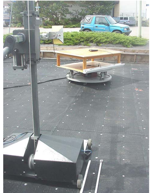
Photograph C.7-4 - Horn Substitution Setup
