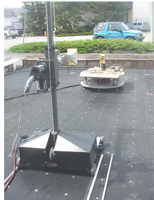
Photograph C.7-4 - Horn Substitution Setup
