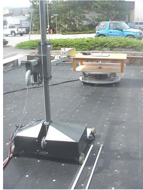
Photograph C.7-8 - Horn Substitution Setup
