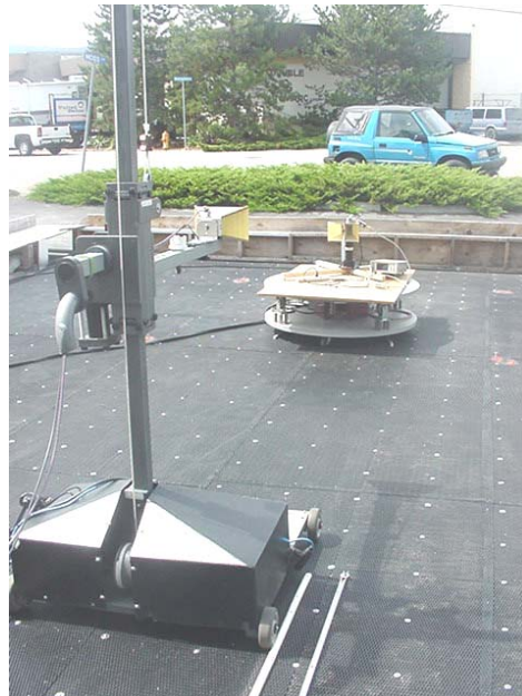
Photograph C.7-8 - Horn Substitution Setup
