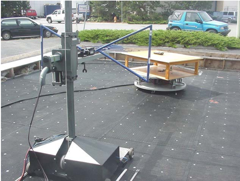
Photograph C.7-3 - Dipole Substitution Setup
