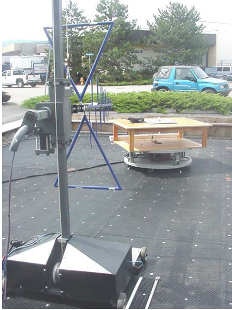
Photograph C.7-7 - Dipole Substitution Setup
