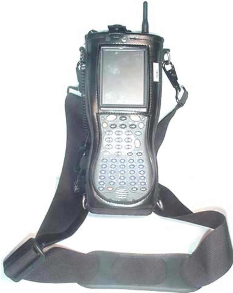
IX100X Handheld PC with Carry Case and Shoulder-Strap accessory (P/N: 77041A) (with JABRA Ear-Microphone accessory)
