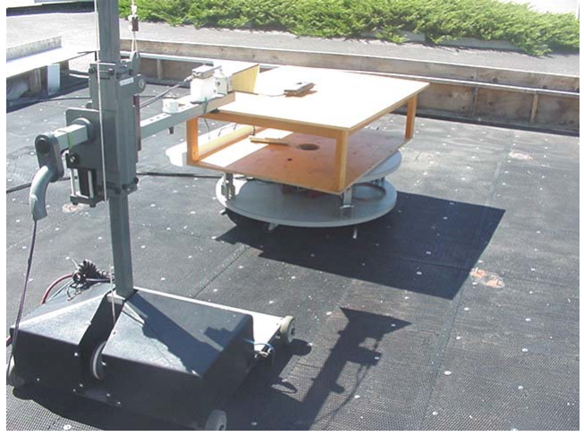
Photograph D.7-2 - Horn Receive Antenna with IX100X and MaxRad Vehicle-Mount Antenna Configuration
