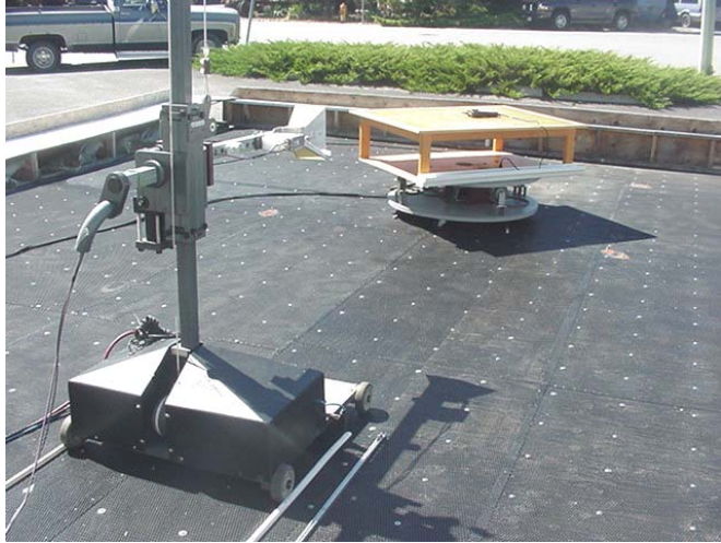
Photograph D.7-1 - BiConilog Receive Antenna with IX100X and Nearson Helix Antenna Configuration
