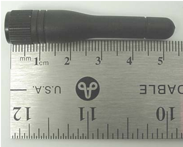
Dual-Band GPRS Antenna - 1/4 wave Helix
