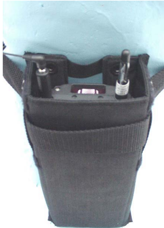
Back Side of DUT facing body - worst-case antenna configuration relative to left torso
