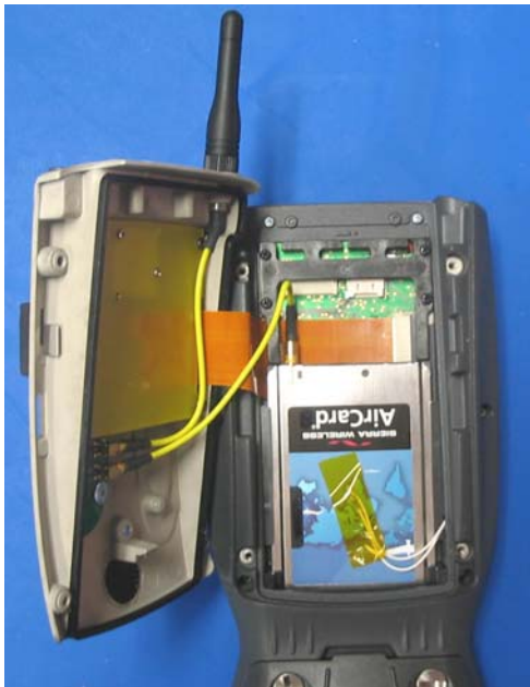
Photograph A.1-3 - IX100X Rugged Handheld PC with AirCard 775 GSM GPRS/EDGE Modem
