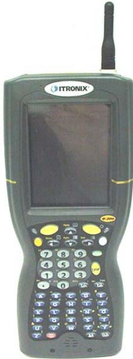
Photograph A.1-3 - IX100X Rugged Handheld PC with AirCard 775 GSM GPRS/EDGE Modem
