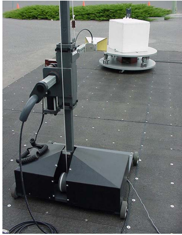
Photograph D.7-2 - Horn Receive Antenna with DUT Helix Antenna Configuration
