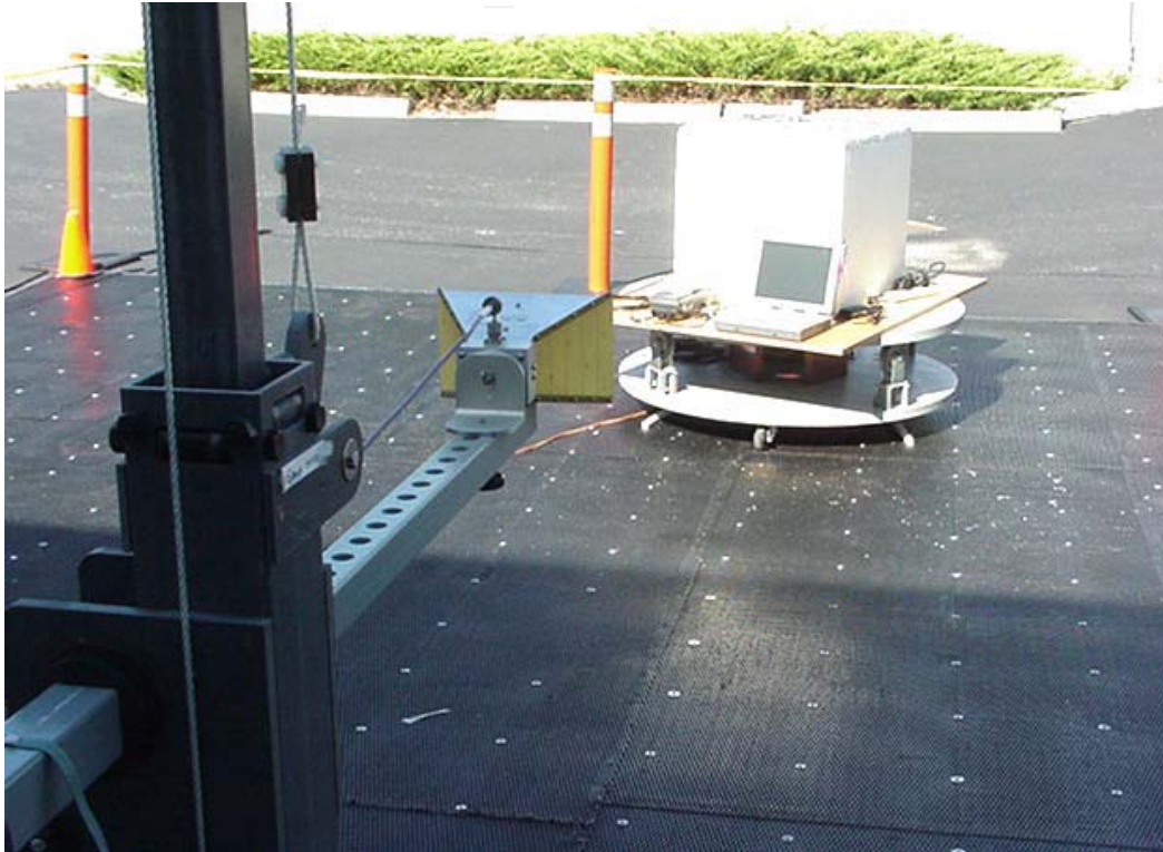
DUT with Vehicle Cradle & MaxRad 3 dBi Gain Vehicle-Mount Antenna (P/N: WMLPVDB800/1900)
