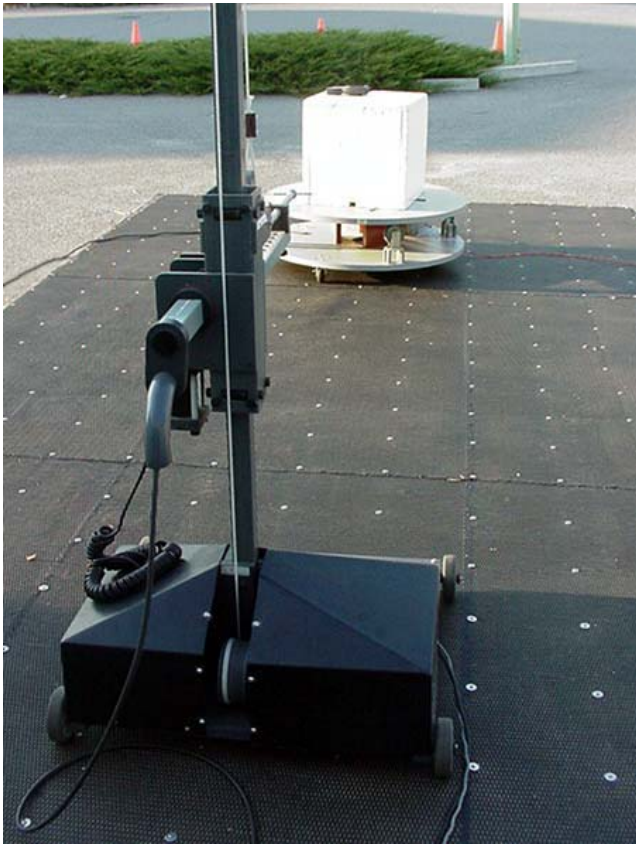
Cellular Band - Dipole Receive Antenna - Horizontal Polarization
