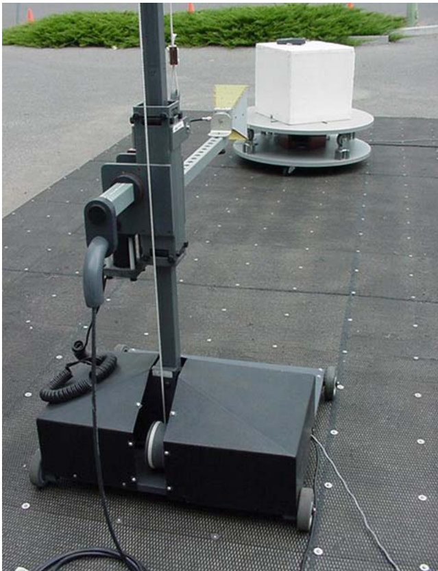
PCS Band - Horn Receive Antenna - Horizontal Polarization
