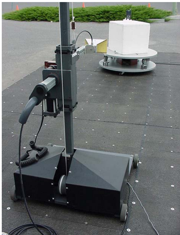
Photograph D.7-1 - Horn Receive Antenna with DUT Helix Antenna Configuration
