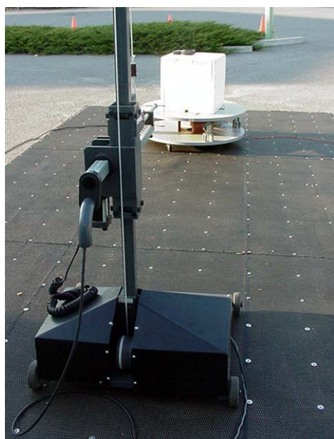
Photograph C.7-3 - Horn Receive Antenna with DUT Vehicle-Mount Antenna Configuration
