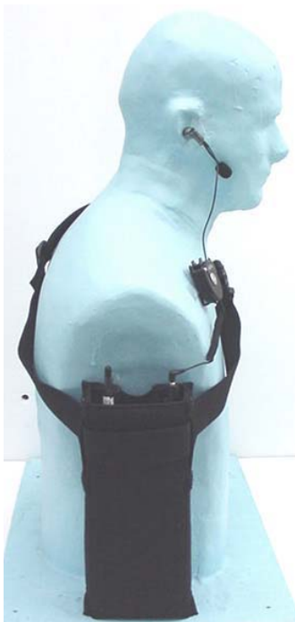
Front Side of DUT facing body - worst-case antenna configuration relative to right torso
